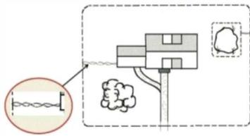
Place the transmitter in a dry, well ventilated area and then plan and lay out the boundary wire that best suits your property boundary. The boundary wire must be a single continuous loop starting and finishing at the transmitter box.
