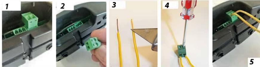
To connect the boundary wire into your transmitter, locate the 2 holed block in the bottom of the transmitter (above 1), remove the green block (above 2), strip back the yellow plastic to expose the copper wire of each wire (above 3). Insert both copper ends and tighten screws with Flathead screwdriver (above 4). Finally, put the complete wired up block back into the original position in the transmitter (above 5).
